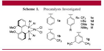
(1a-g, Scheme 1). The reaction of methylenecyclohexane and ethyl glyoxylate (eq 1, Table 1) was chosen for testing.
